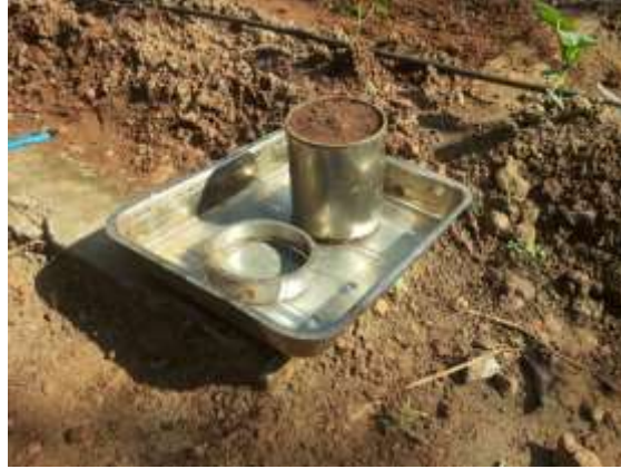
Plate 3.1 Determination of bulk density by core cutter
