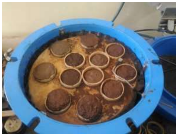
Plate 3.3 Soil samples in pressure plate and membrane apparatus
