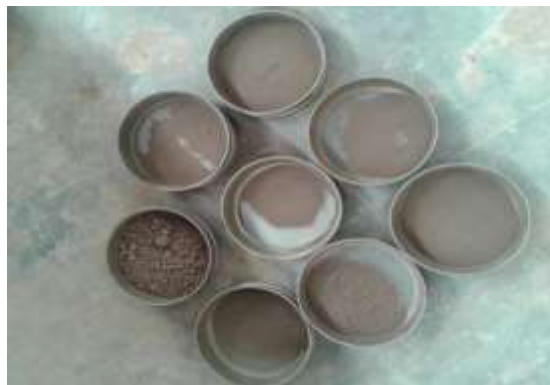
Plate 3.2 Soil retained on different sieves
