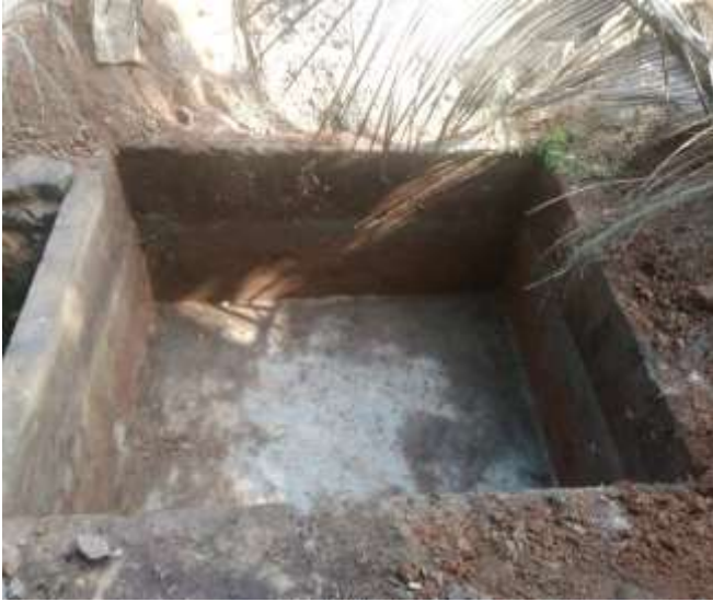
Plate 3.4 A view of lysimeter tank
