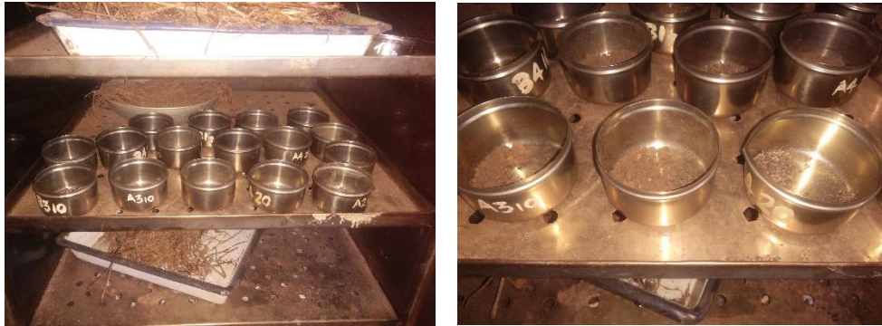
Plate 3.11 Moisture content estimation by oven drying method
