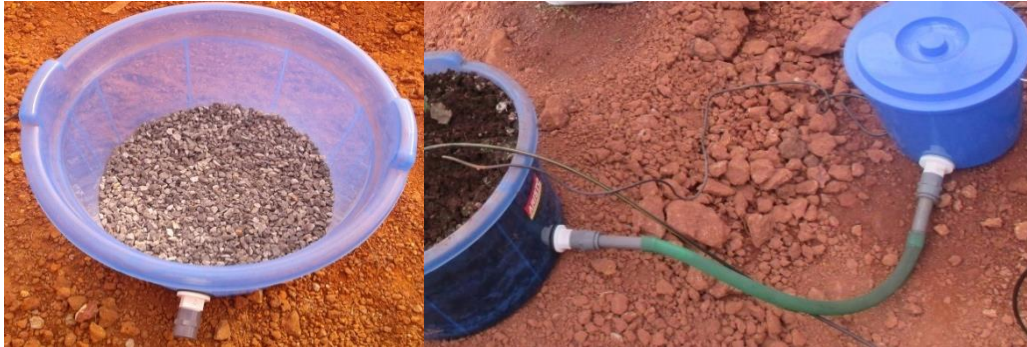
Plate 3.4 Non-weighing Mini lysimeter with drainage system
