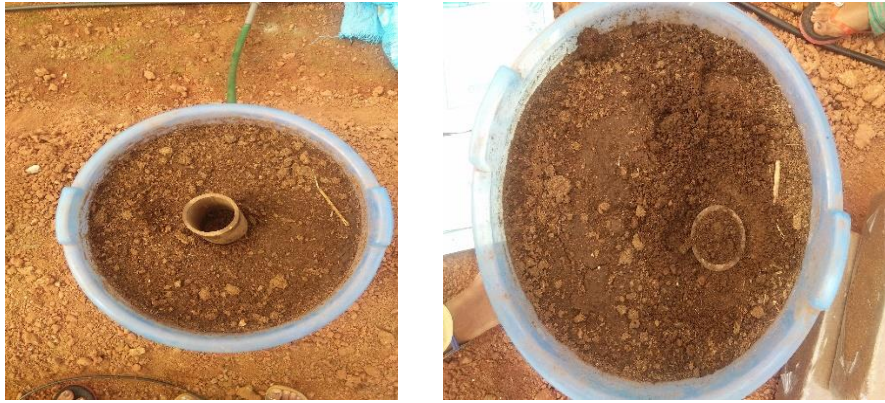
Plate 3.1 Determination of Bulk density by Core cutter
