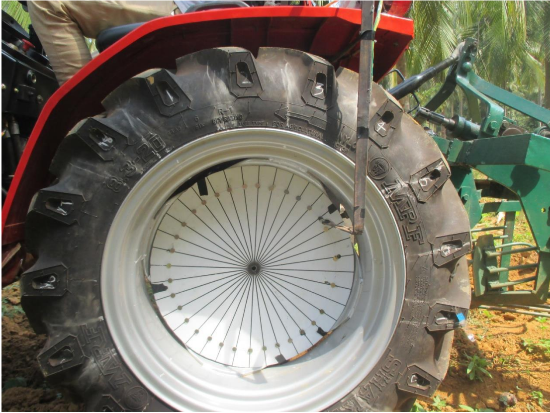
Plate 4.2 working of slip meter under load condition
