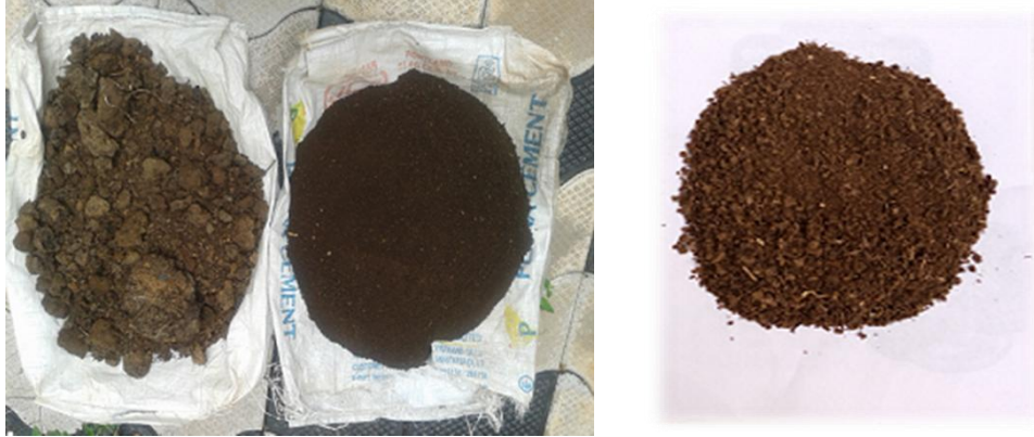
Plate.4.1 cow dung powder observed from 5 mm and 10 mm IS sieves
