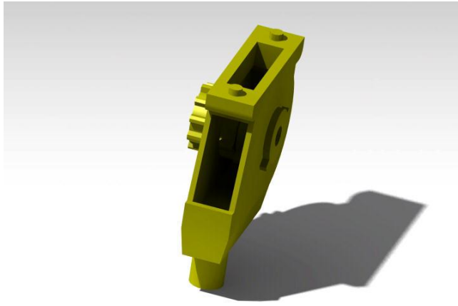
Fig. 3.9 3D CAD image of fluted roller
