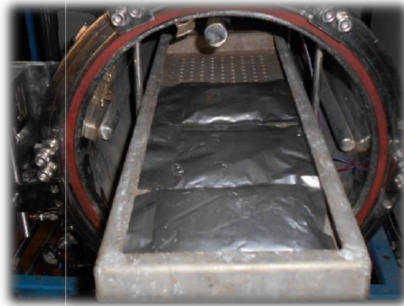
Plate 3.5 Filling of pouches in retort
