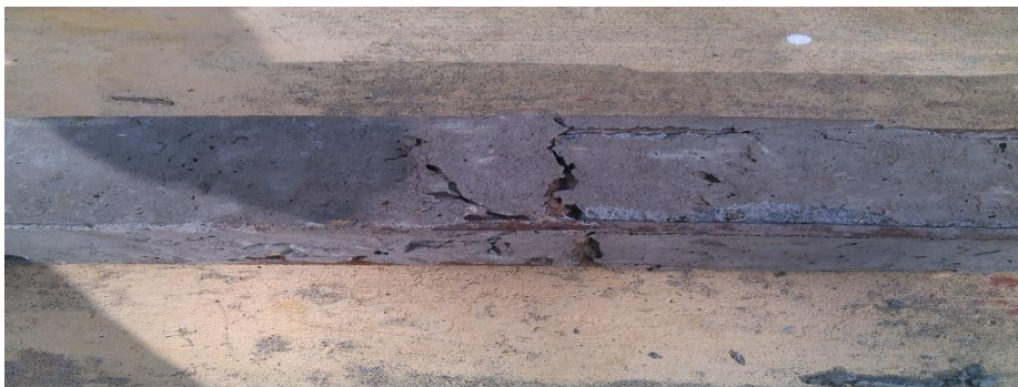
Figure 21-Concrete post after bending test
