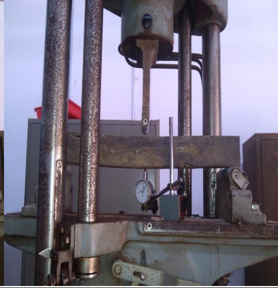
Figure 19- RPL subjected to bending test
