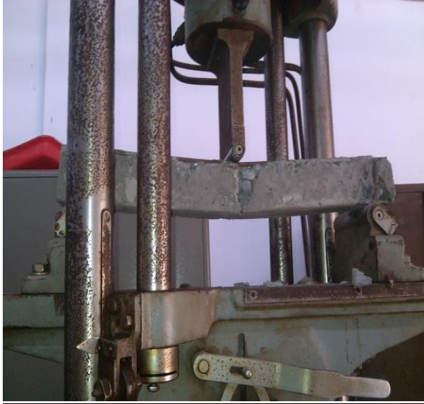
Figure 18-Concrete post subjected to tension
