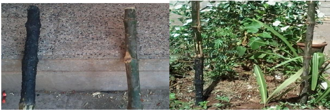
Figure 15-Plastic coated bamboo and normal bamboo pole
