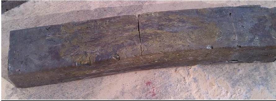
Figure 20-RPL after bending test
