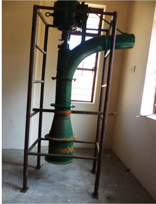
Plate.3.1 Laboratory model of the axial flow propeller pump
