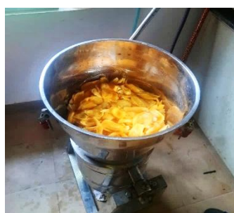
Plate. 3.2 Jackfruit pulping using industrial mixer
