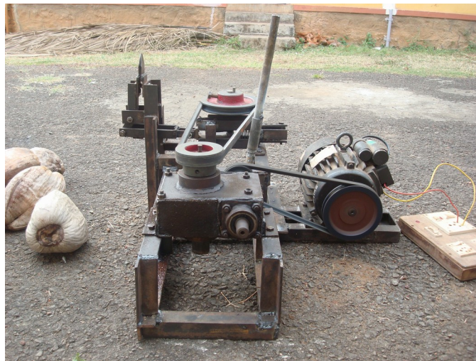
Fig. 3.8.b. Powered-coconut husking machine ( Side view )
