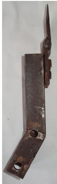
Fig. 3.7 Angular 2-arm lever with blade (Side View)
