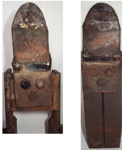
Fig. 3.6 Fixed blade and movable blade
