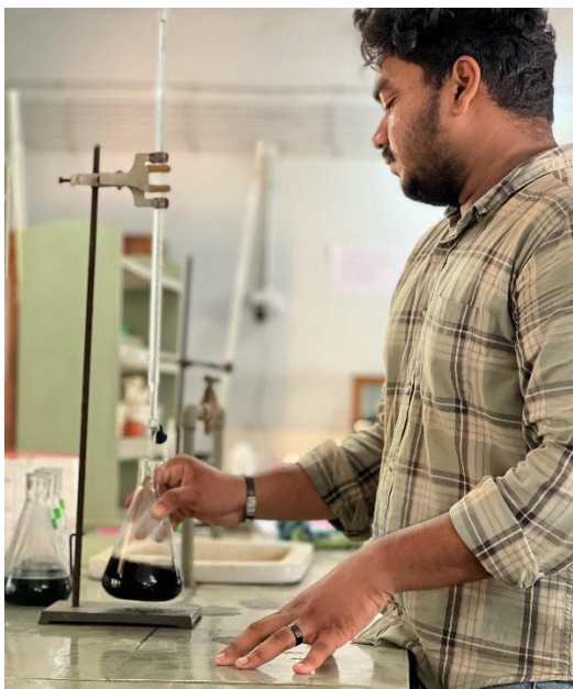
Plate.3.4 Testing of organic matter content in soil
