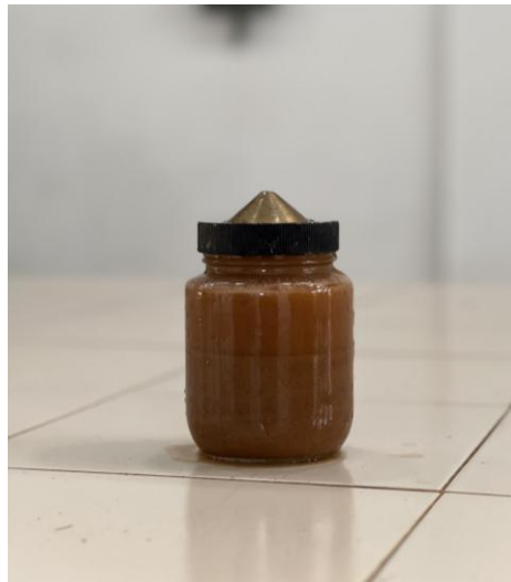
Plate.3.2 Pycnometer for Specific Gravity determination
