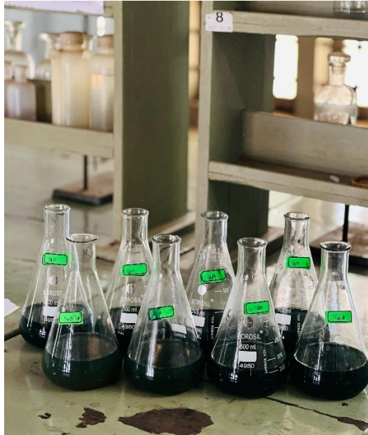
Plate.3.4 Testing of organic matter content in soil
