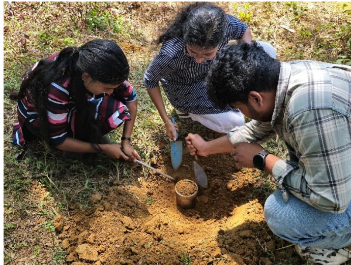
Plate.3.1 Sample collection for determining bulk density
