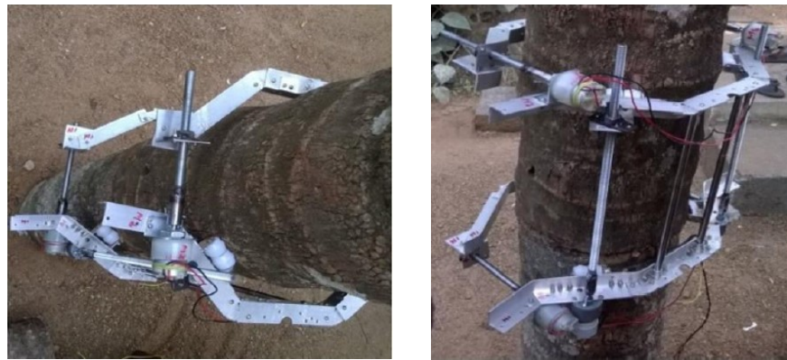
Fig. 2.23 Top view and front view of harvesting device (Dubey et al. , 2016)
