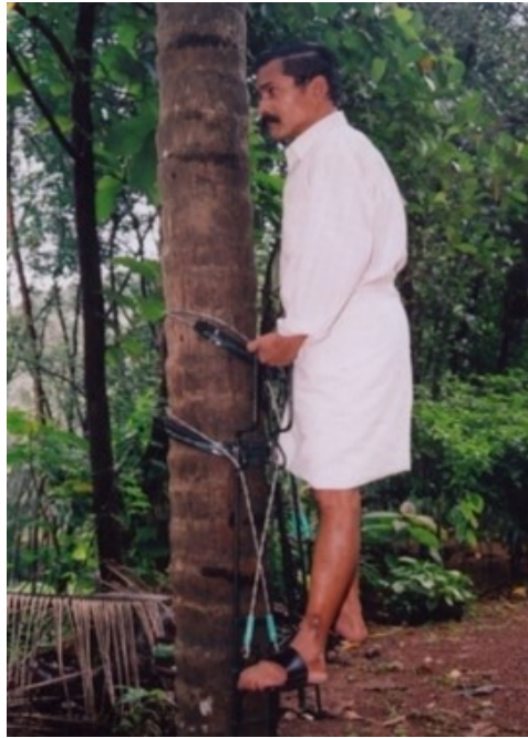
Fig.2.11. Chemberi model coconut climbing device (Anand, 2014)
