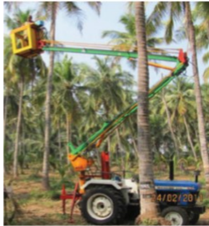
Fig. 2.20 Tractor mounted and self-propelled coconut climber for coconut harvesting (Kolhe, 2014)
