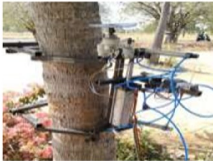
Fig. 2.25 Pneumatic coconut tree climber and harvester (Dinesh and Muthukumar, 2020).
