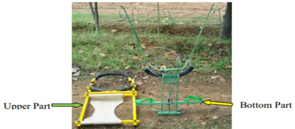
Fig. 2.18 Modified coconut climbing device (Sridhar et al. , 2017)
