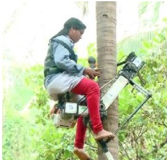
Fig. 2.21. Man carrying bike developed by M/s Mabens Engineering Solutions, Shimoga
