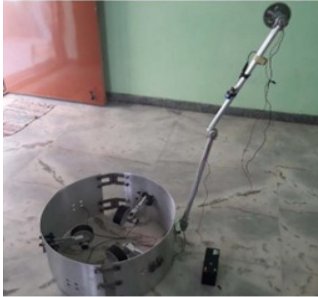
Fig. 2.24 Automated coconut tree climbing device (Azarudeen et al. , 2018)
