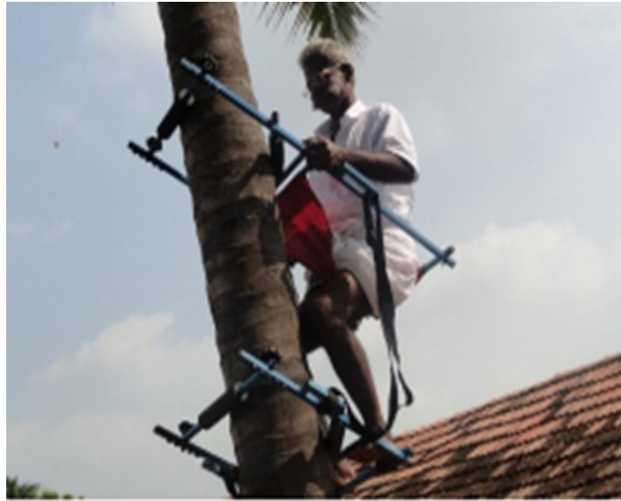
Fig. 2.13. TNAU model climbing device (Krishnan et al , 2013)
