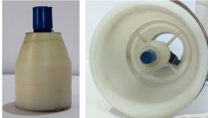
Plate 4. Arrangement of spray nozzle inside the spray gun
