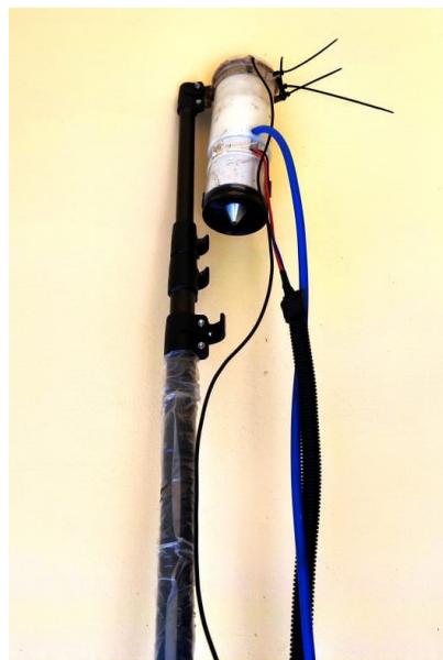
Plate 5. Spray gun mounted at the top end of telescopic pole
