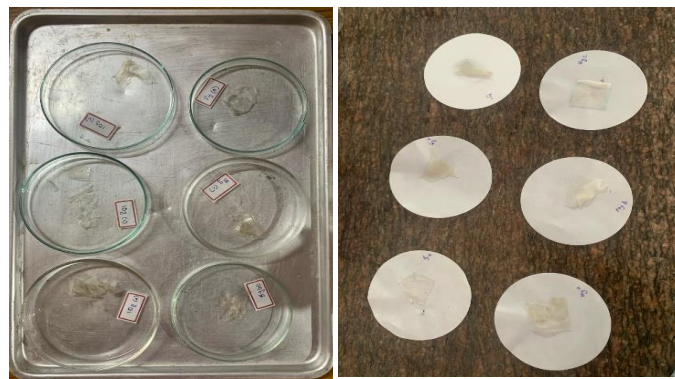
Plate 3.10 Solubility and swelling index of biodegradable film
