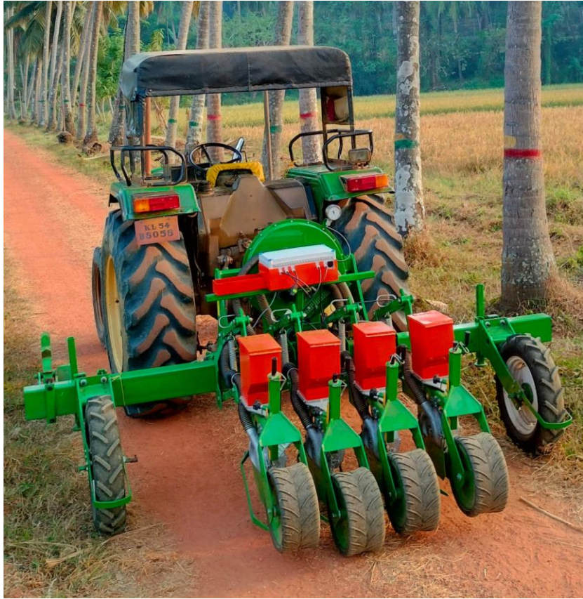
Plate 3.25 Developed tractor operated pneumatic no-till pulse planter with electronic control system
