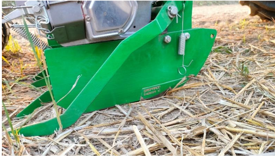
Plate 3.22 Stub type runner and seed covering device
