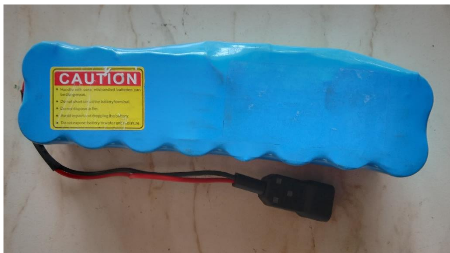
Plate 3.13 Lithium iron phosphate battery
