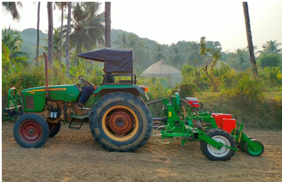
Plate 3.26 Working of pneumatic planter with electronic control system
