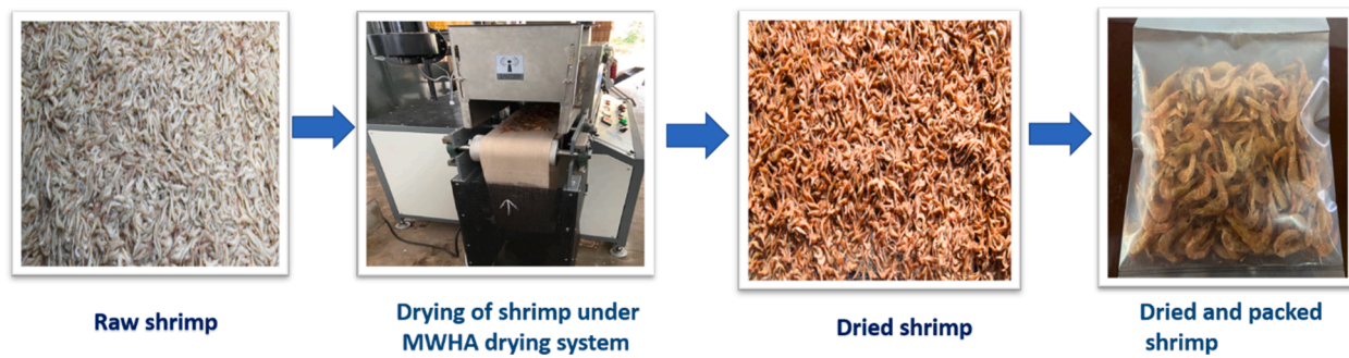
Fig. 2. Drying of shrimp under microwave drying system.
