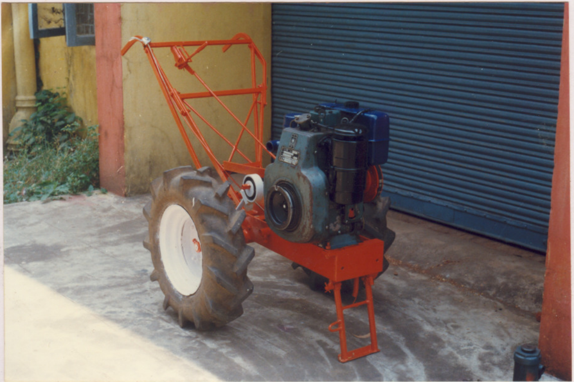
Plate I Front view of Garden Tractor
