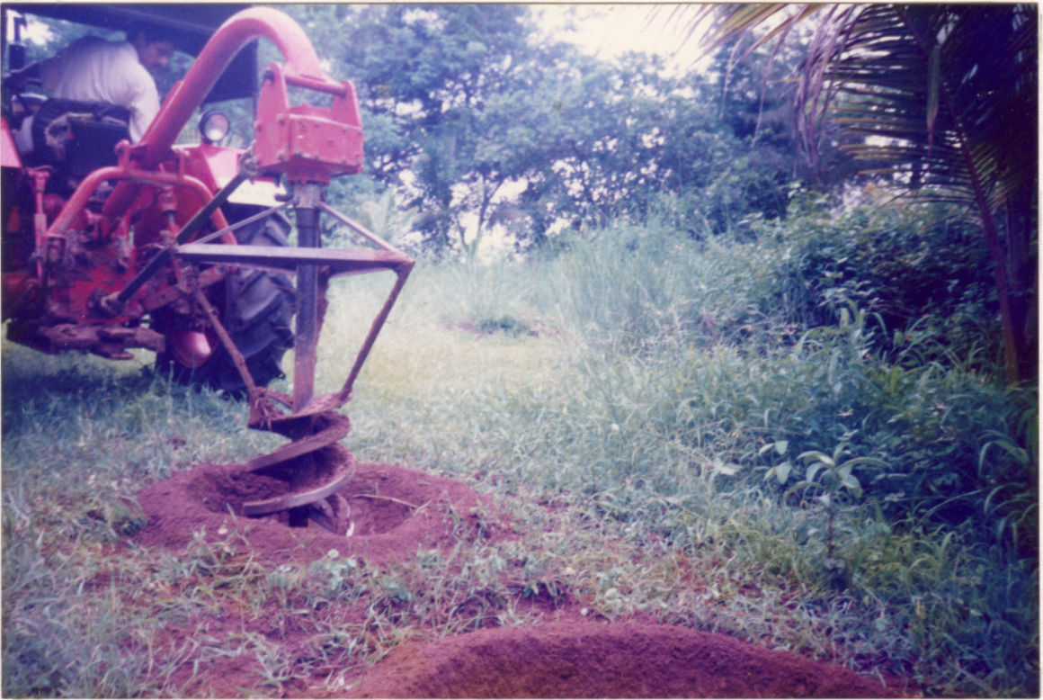
Plate 3.3. Tractor operated post-hole digger with countersinking attachment during field operation (Unit I)
