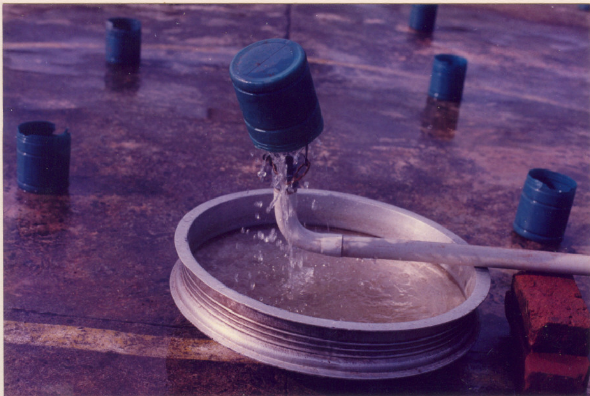
PLATE 5 - MEASUREMENT OF DISCHARGE
