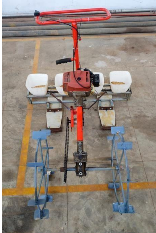
Plate 4.1 Developed self-propelled paddy seeder
