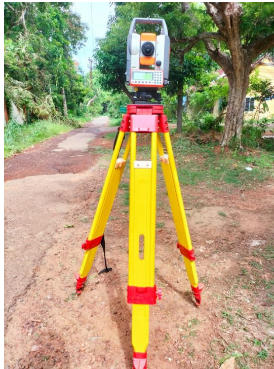
Plate 3.2. A view of Total Station
