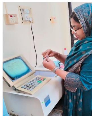
Plate 3. 8 Analysis of Available Phosphorous using UV Spectrophotometer
