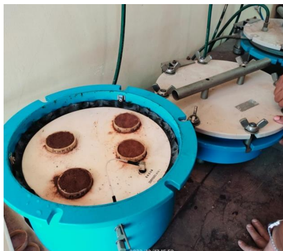
Plate 3. 10 Soil samples in pressure plate apparatus
