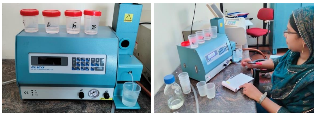
Plate 3. 9 Analysis of Potassium using Flame Photometer
