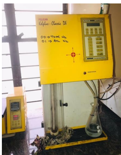
Plate 3. 7 Analysis of Available Nitrogen using Kelplus Nitrogen Analyser
