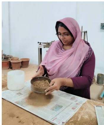
Plate 3. 3 Sieving of air dried soil samples through 2mm sieve
