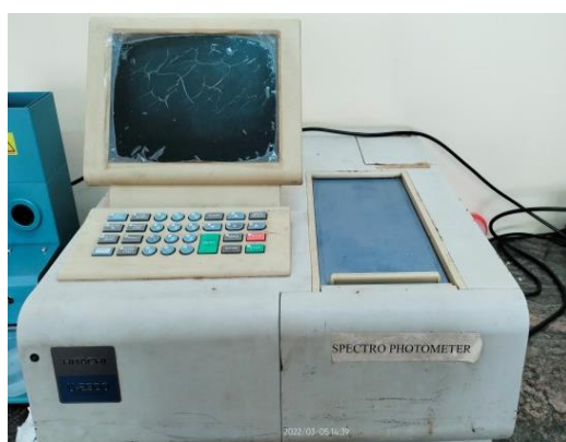
Plate 3. 8 Analysis of Available Phosphorous using UV Spectrophotometer
