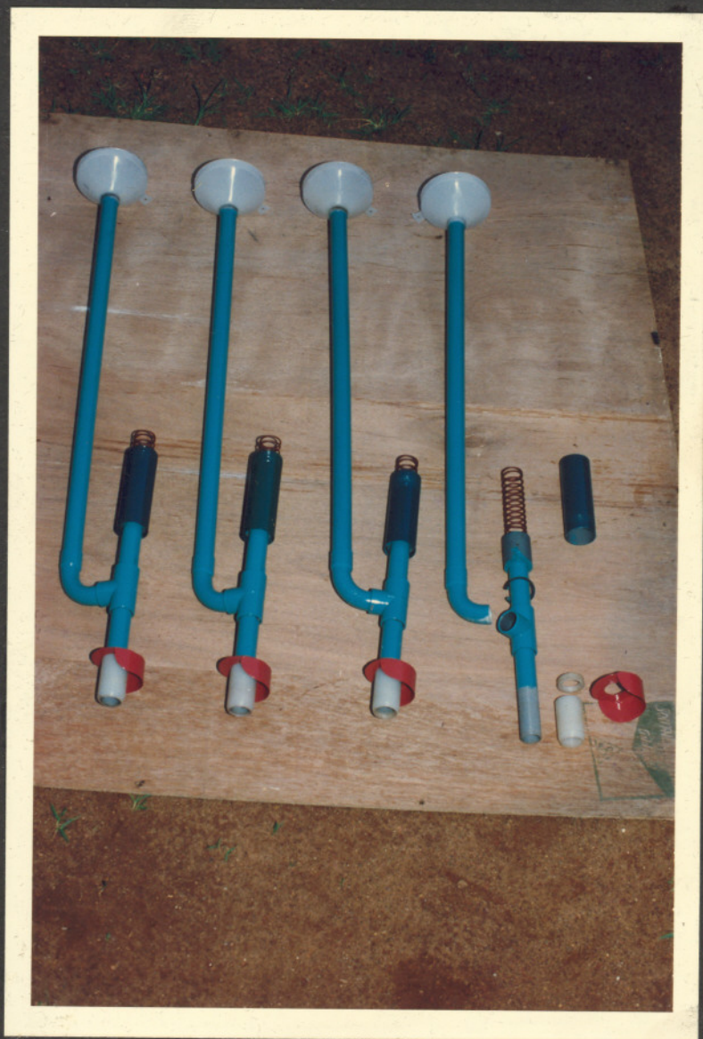
PLATE No.3. DELIVERY TUBE ASSEMBLY AND ITS EXPLODED VIEW.
