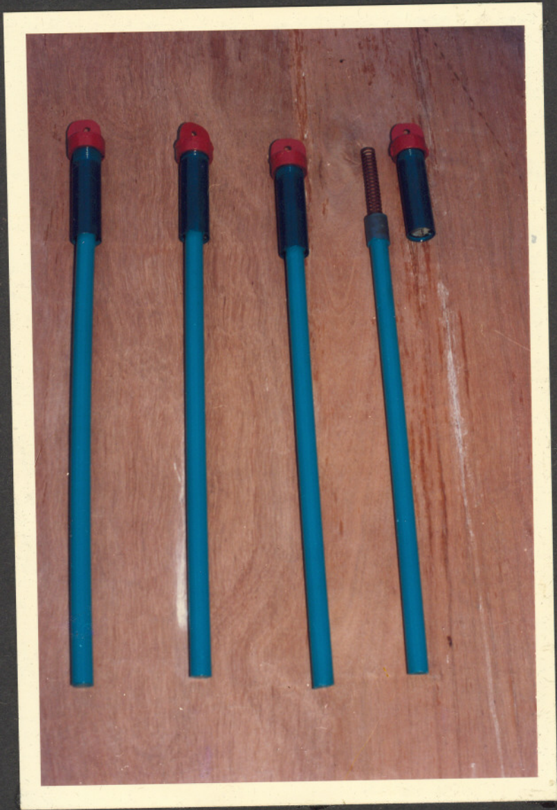
PLATE No.2. PLUNGERS AND ITS EXPLODED VIEW.
