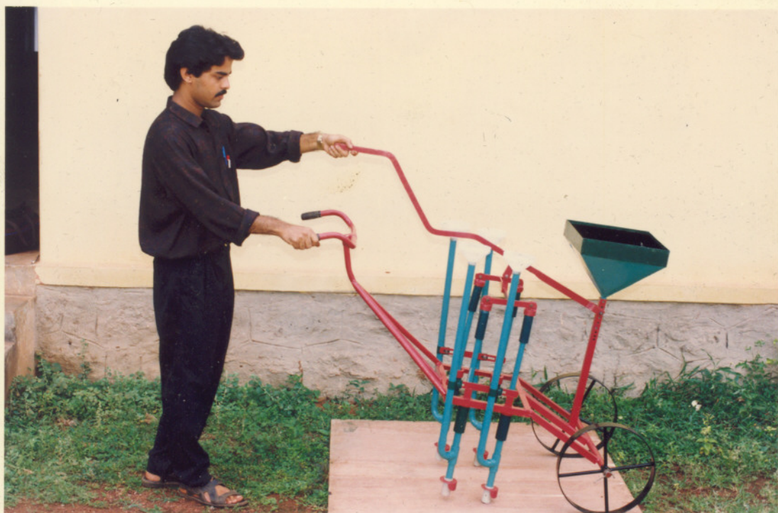
PLATE No.6(b) . OPERATING LEVER IN WORKING CONDITION.
