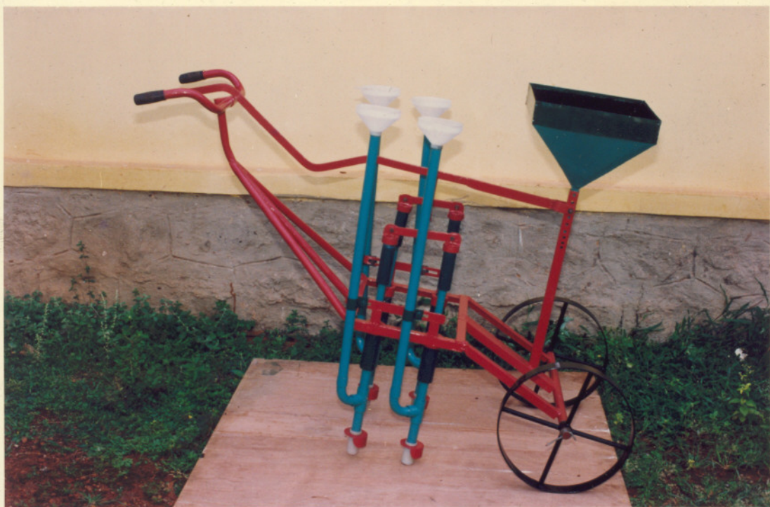
PLATE No.6(a) . SIDE VIEW OF USB APPLICATOR
