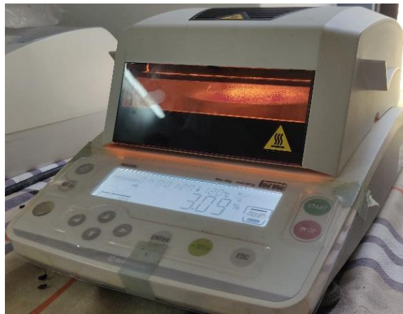
Plate 3.1: Determination of moisture content by infrared method
