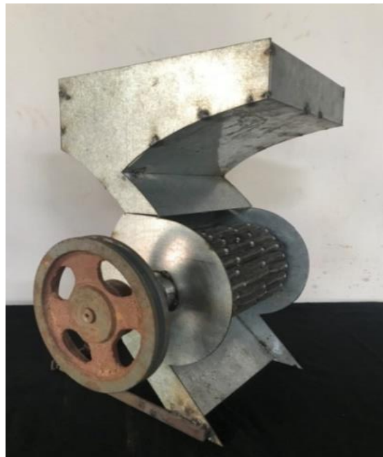
Plate. 3.3: Cocoa bean sheller – The first model
