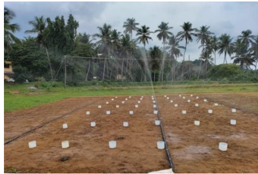
Plate 16. Catch can experiment
