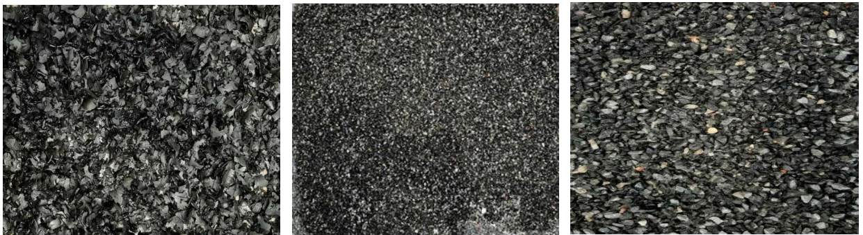
Plate.3.2 Layers of gravel, metal chips and charcoal in secondary chamber - expt I
