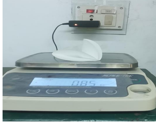
Plate.3.20 Weighing of filter paper
