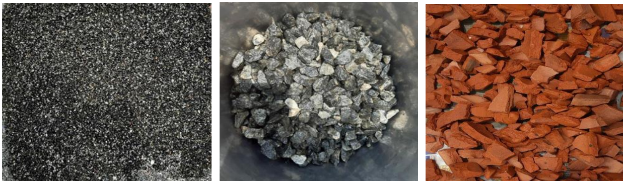
Plate.3.1 Layers of gravel, metal stone and clay roof tile in primary chamber - expt I
