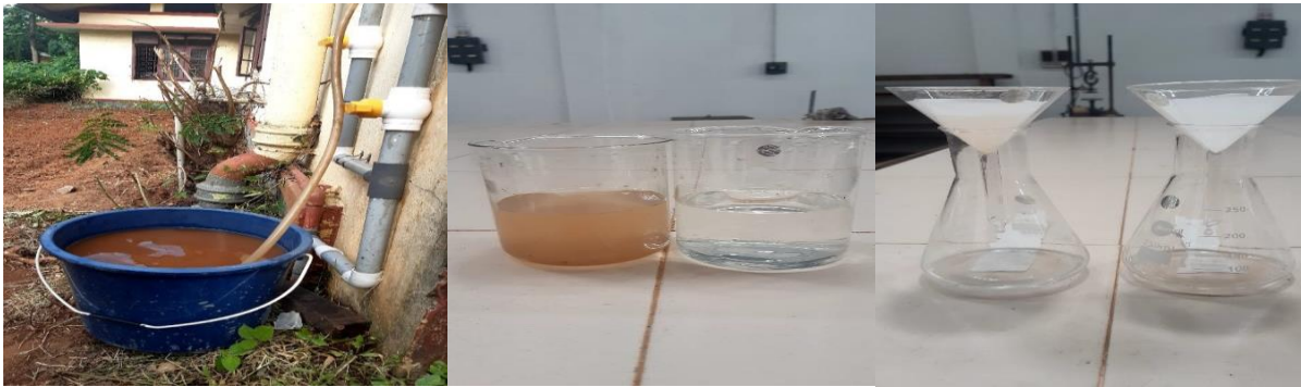
Plate.3.18 Application of muddy water and evaluation of the collected sample
