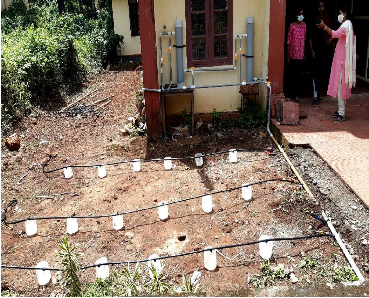
Plate.4.2 Testing of filter for emitter flow
