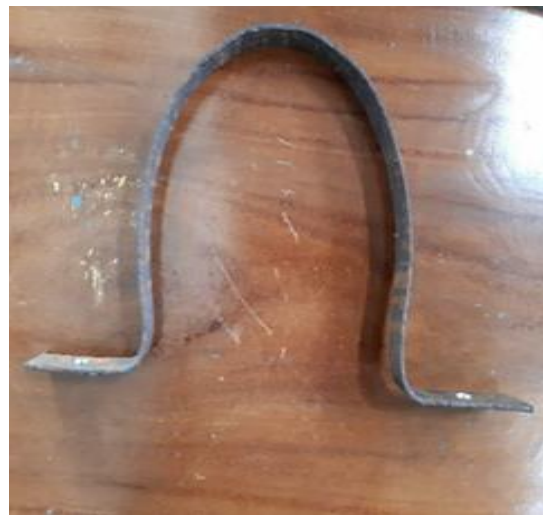
Plate.3.11 Fixing of filter chamber on wall using clamps
