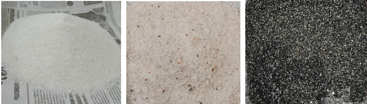
Plate.3.3 Layers of fine sand, silex sand and gravel in primary chamber - expt II
