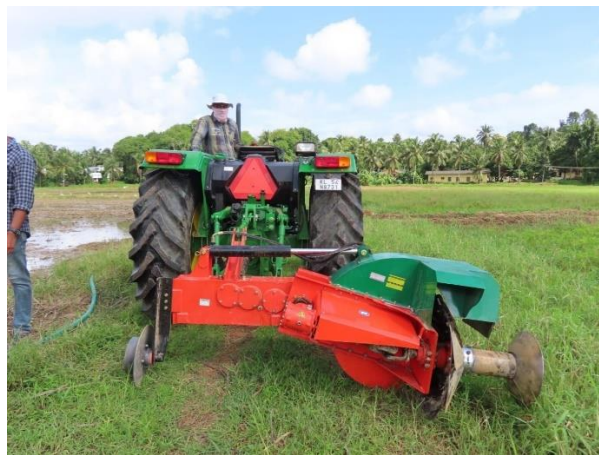
Fig 3.6. Yarrow Farms ridge plastering machine
