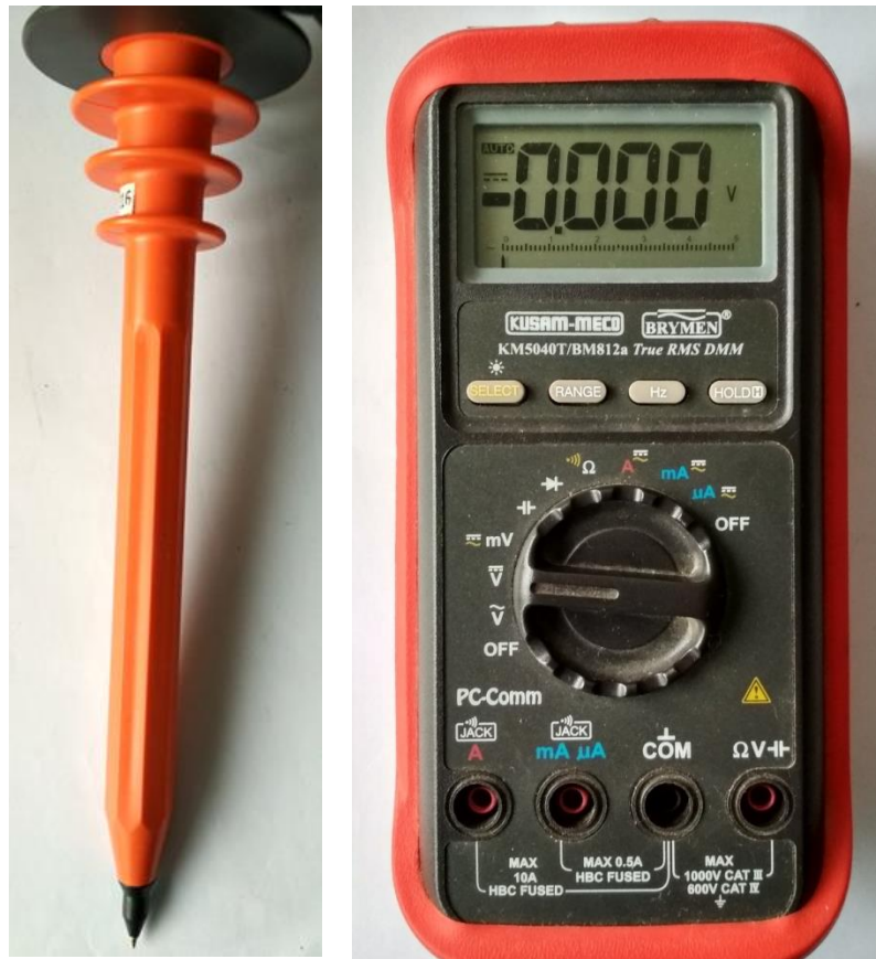
Fig. 3.12. High voltage probe and digital multi-meter
