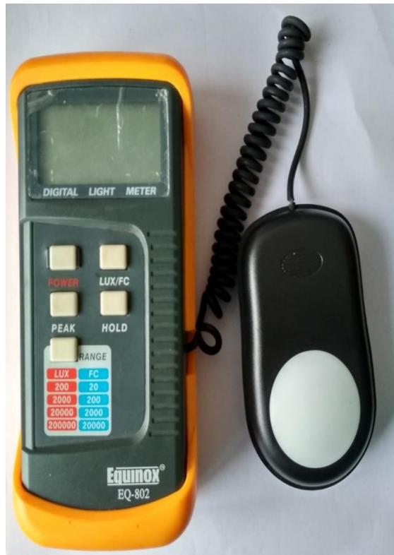
Fig. 3.5. Digital illuminance meter with photon detector
