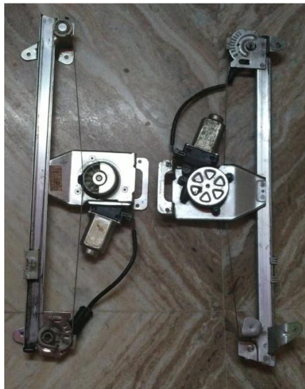
Fig. 4.13 DC motor operated cable drive slider mechanism
