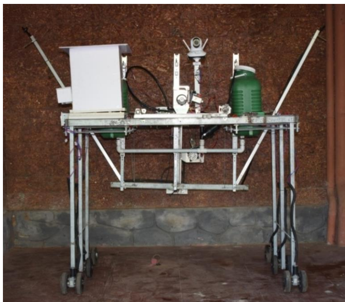
Fig. 4.23 Developed prototype of semi-autonomous robotic platform
