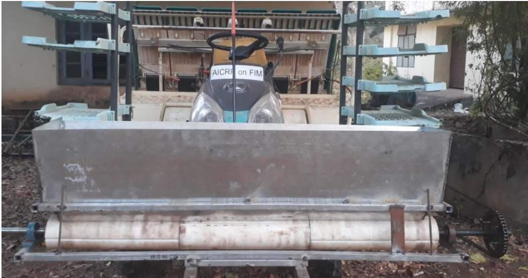
Plate 4.2: Fertiliser box being attached to the transplanter
