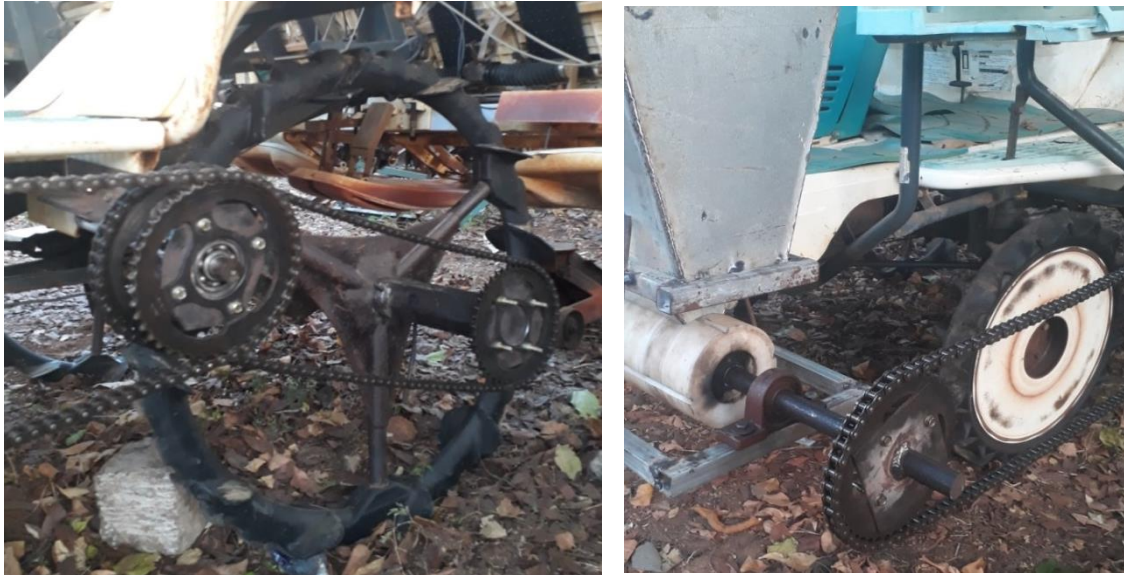
Plate 4.1: Power transfer mechanism fabricated in the KUBOTA rice transplanter
