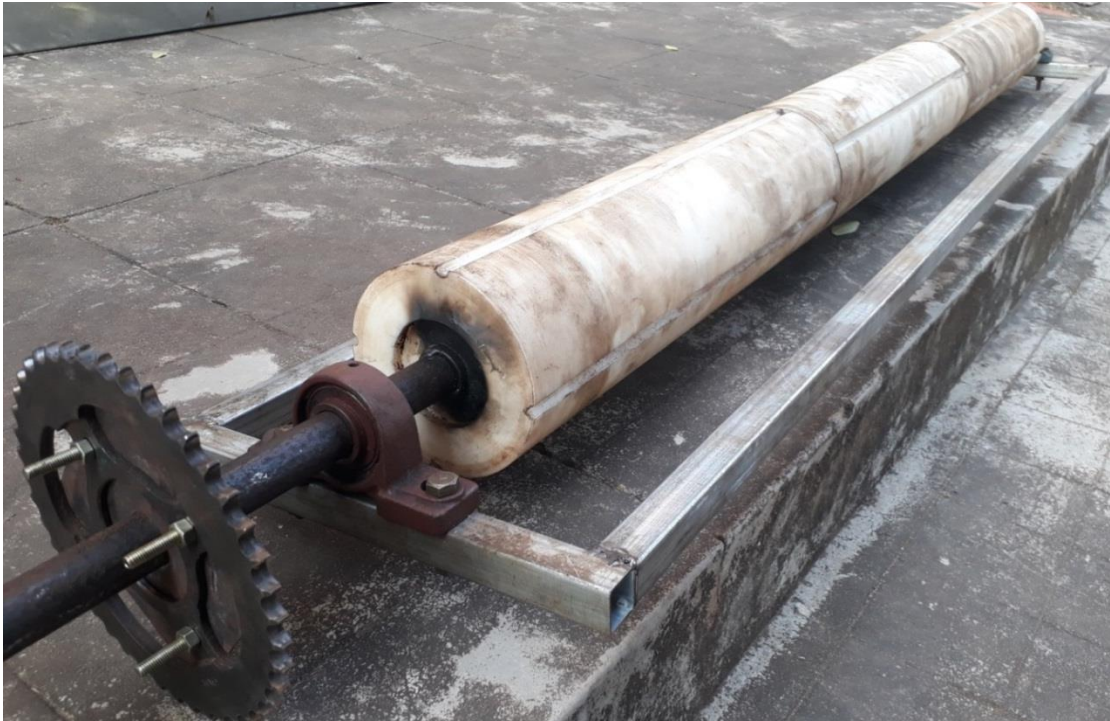
Plate 4.3: Fabrication of metering unit with power transferring sprocket and shaft
