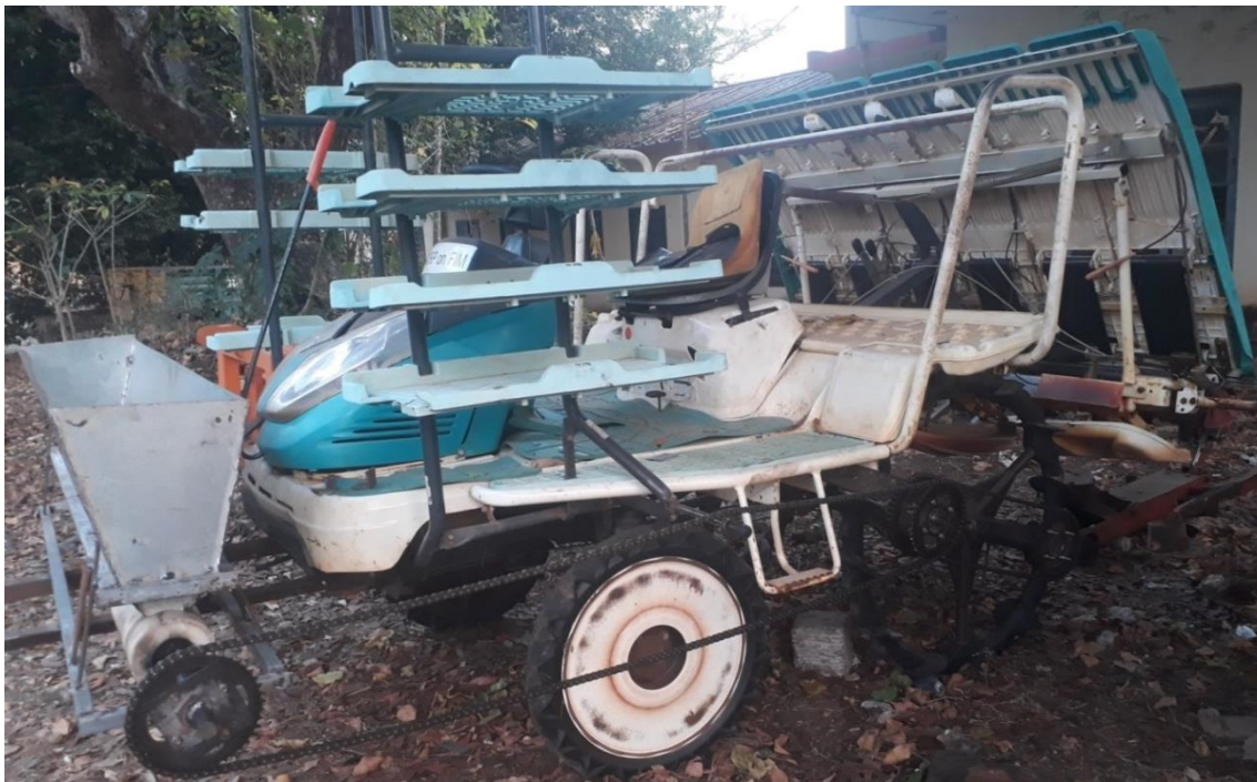
Plate 4.4: Developed fertilizer metering device for the transplanter
