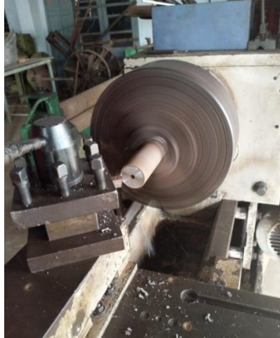
Plate 3.12 Turning of shaft in lathe
