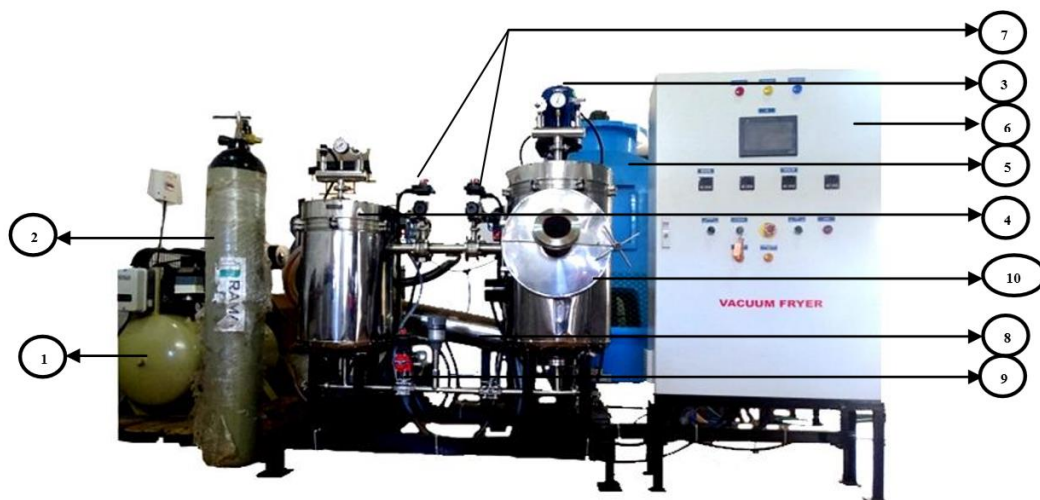
Plate 3.2. Developed Vacuum Frying System (KCAET, Tavanur, Kerala)
