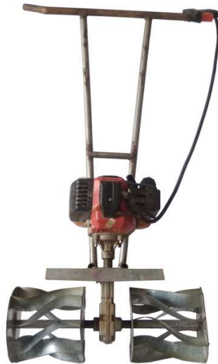
Figure 4.17 Helical blade rotor attached to MPTC
