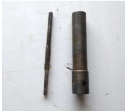
Figure 4.5 Power transmission shaft with hollow casing
