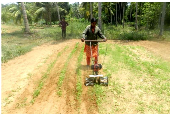
Figure 4.33 Testing of surface pulveriser cum two-row vegetable weeder
