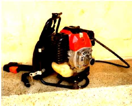
Figure 3.4 Engine of back pack type brush cutter
