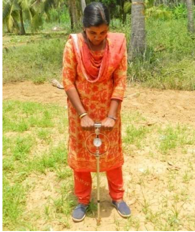
Figure 3.2 Measurement of Cone index
