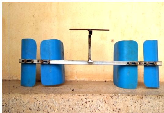
Figure 4.12 Plastic guards fixed with GI frame
