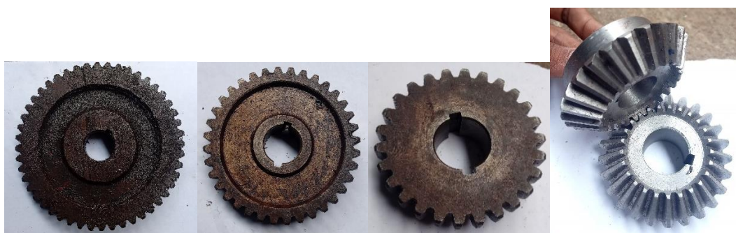
Plate 3.15 Spur gears and bevel gears
