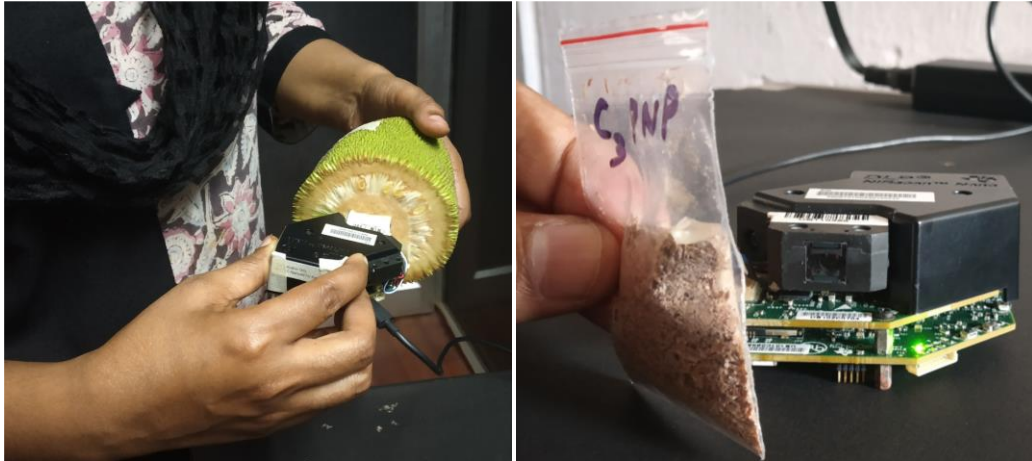
Plate C2. Spectra acquisition using DLP NIRscan Nano
