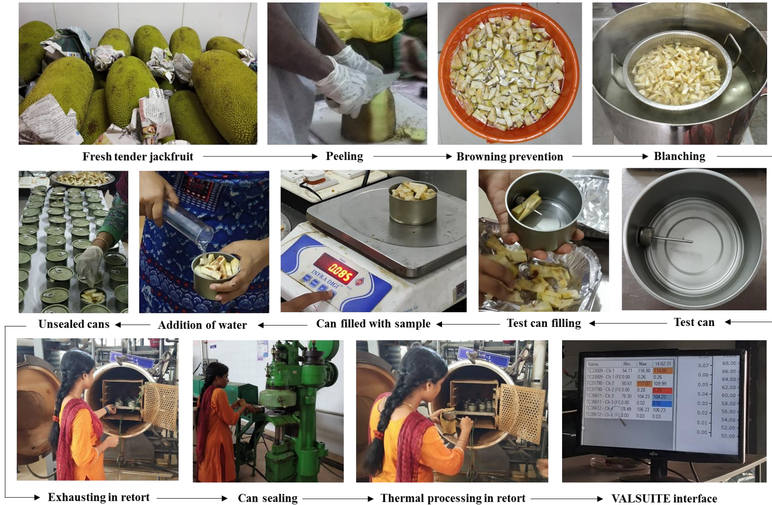
Fig. 3.1 Steps involved in thermal processing and canning of tender jackfruit
