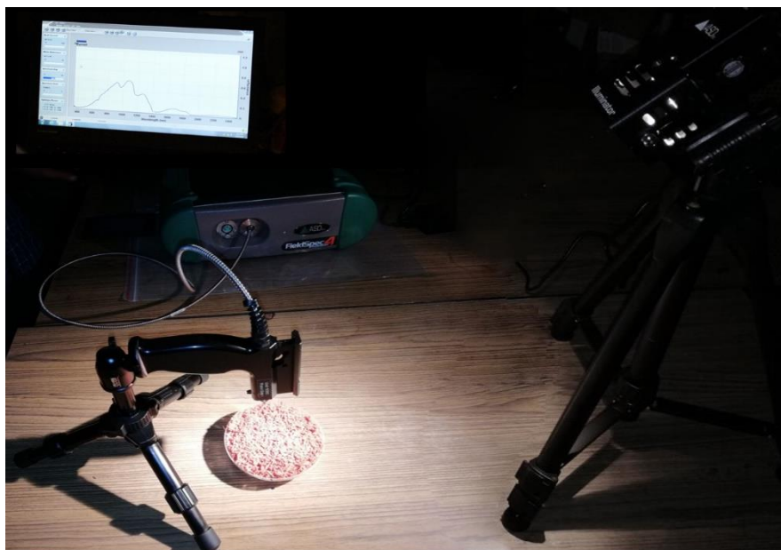
Plate C1. Spectra acquisition using ASD FieldSpec-4 spectroradiometer
