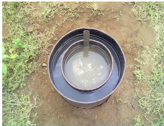
Plate 10 Double ring infiltrometer set up in the field
